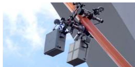
Figure 1. Cable-stayed bridge (Tomei Ashigara Bridge) Figure 2. Self-propelled stay-cable inspection device
